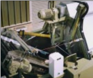
Barrel door and outfeed elevator incorporating safety cord
