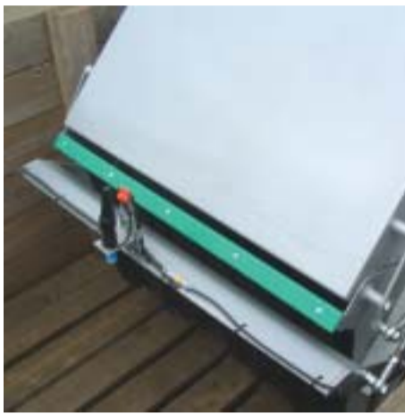
Ultrasonic crop sensor with self-adjusting bracket for consistent crop detection
